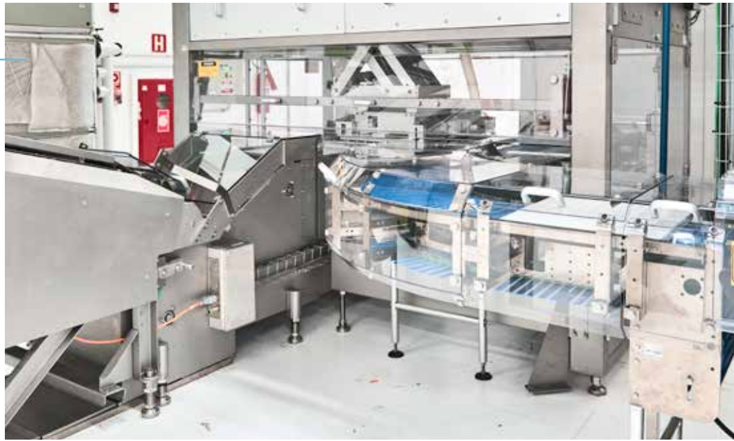
Biscuit feeding by HiFlex robot with linear motor drive
