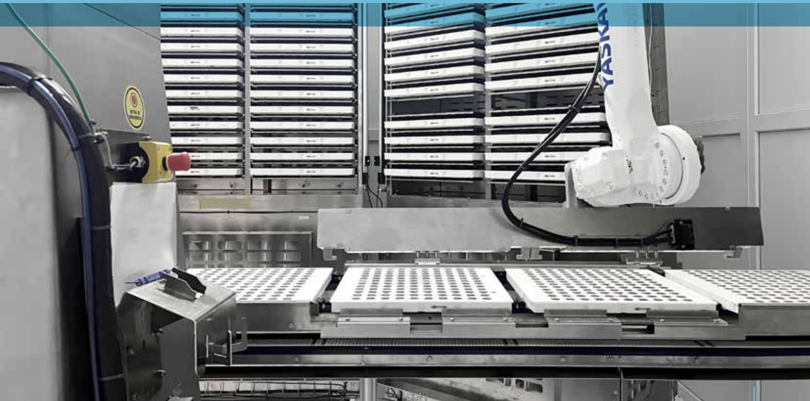
Yaskawa GP50 robot places mould pallets in assigned slots in the robot cooling cell
